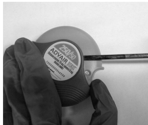
Figure 2: Removal of outer shell
