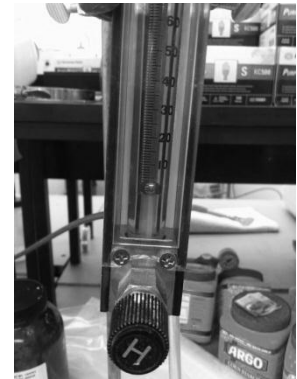
Figures 3 and 4. From left to right; the inlet air valve and the flow meter used in the fluidized bed setup.
