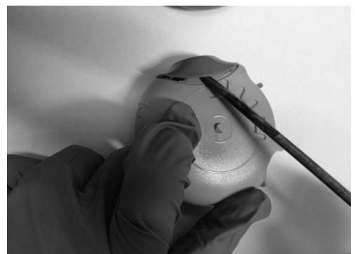
Figure 3: Proper removal of mouthpiece
