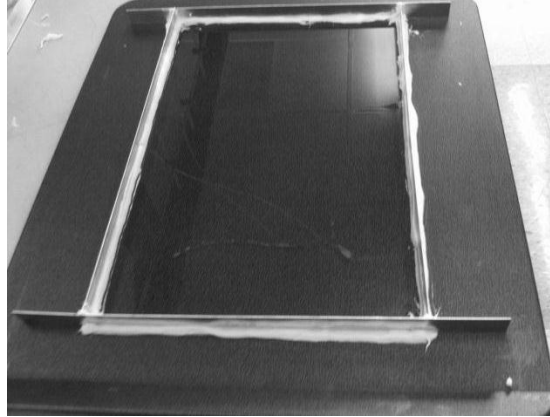
Figure 16. The casting tray used to create dissolvable strips. The surface is a Teflon ® baking sheet, and the guides are aluminum strips. The guides are reinforced using silicone caulk.
