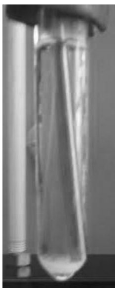
Figure 9. The DXM and water solution once recrystallization has begun. Notice the white substance at the bottom of the tube.
